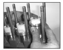
14. Press seal sleeve assembly into the manifold and seat firmly. Put the supportring (41) on plunger with v-side facing the manifold.
